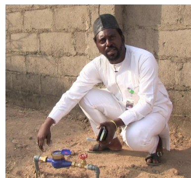
Exhibit 40. TAWASCO testing customer meter functionality in its efforts to reduce commercial NRW.
