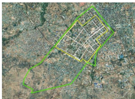
Exhibit 42. NISWASEC established its first-ever Shiroro Tank Pressure Zone and DMA in Minna to help manage NRW and increase financial viability.
