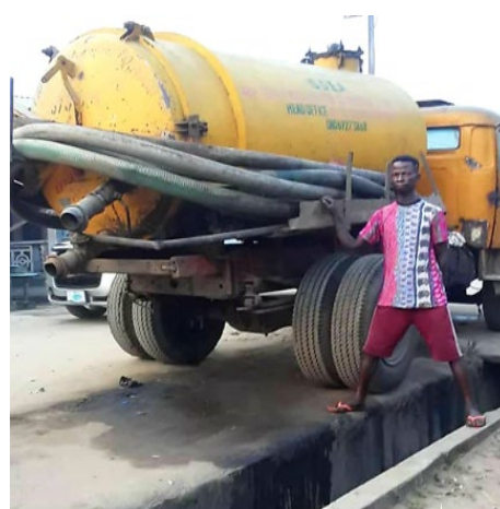
Exhibit 64. Generally, FSM small businesses like this in Owerri, Imo, have 1–2 trucks, while operators do not have personal protective equipment and parts, licenses, or inspection programs.
