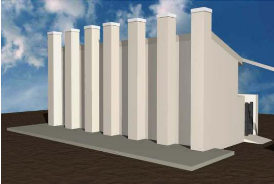
Plate 3.1: Back elevation of the VIP latrine superstructure showing the blockwork vent pipe
